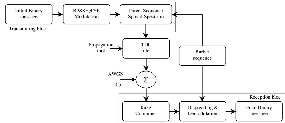
**Fig. 5.** Digital transmission chain
