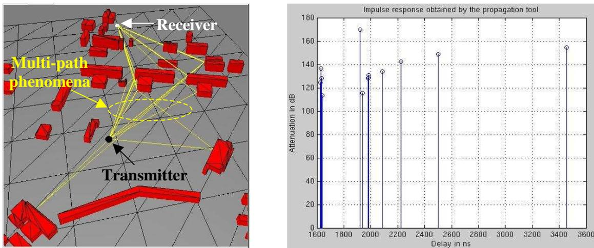
**Fig. 4.** Propagation Tool and channel impulse response obtained
