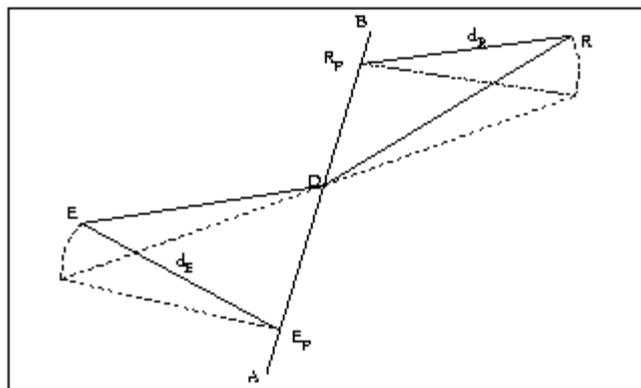
*Fig. 1. Analytical Solution for Computing a Path with One Diffraction Point*
