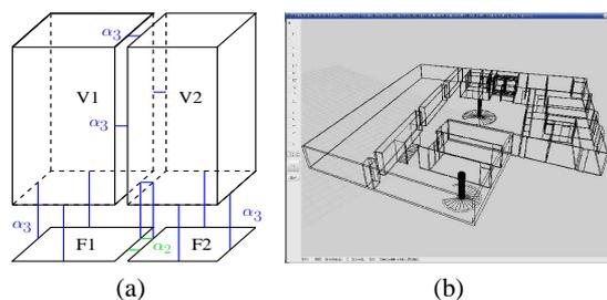
Figure 3: Extrusion of walls: (a) volumes  $V_1$  and  $V_2$  are built and connected to the corresponding faces  $F_1$  and  $F_2$ . Since  $F_1$  and  $F_2$  are connected by  $\alpha_2$ ,  $V_1$  and  $V_2$  are connected by  $\alpha_3$ . (b) sample floor with walls extrusion.
