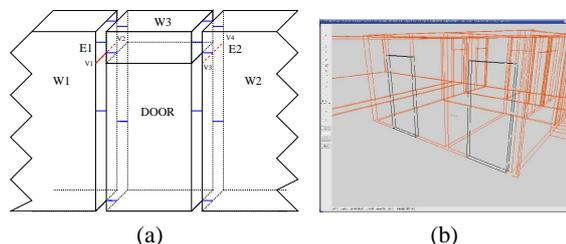
Figure 4: Door extrusion: (a) extrusion and connexion to the walls  $W_1$  and  $W_2$ , the section of wall named  $W_3$  is built above the door. Four vertices ( $V_1, V_2, V_3, V_4$ ) and two edges,  $A_1$  and  $A_2$ , are inserted on  $M_1$  and  $M_2$ . (b) Result of door extrusion.
