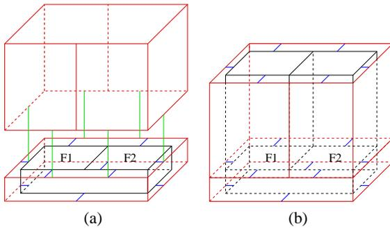
Figure 7: (a) The outer ground volume is sewed by  $\alpha_2$  to the external floor volume (facade); (b) the resulting open volume (in red) represents the floor facade and the ground.
