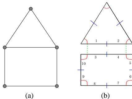
Figure 2: (a) A 2D object containing 2 faces, 6 edges and 5 vertices; (b) corresponding generalized map: the set of darts  $\{1,2,3,4\}$  represents an edge, the set of darts  $\{3,4,5,6,7,8,9,10\}$  represents a face.
